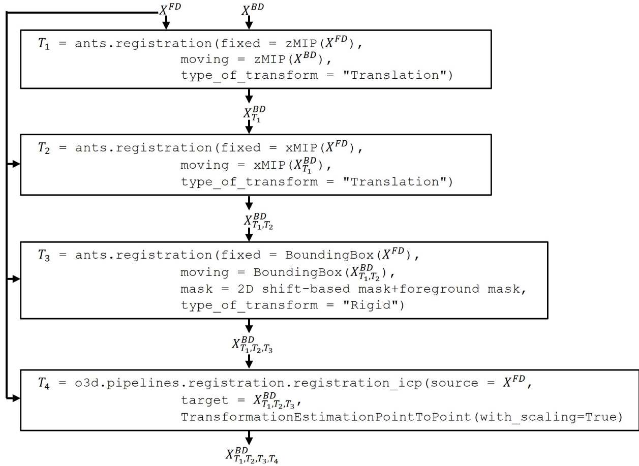
Supplementary Fig. 11. An illustration of the registration workflow in Leonardo, which is based on ANTsPy (ants). From coarse to fine, Leonardo registers input datasets using their maximum intensity projections (along the z-axis, i.e., zMIP, or along the x-axis, i.e., xMIP), 3D downsampled and cropped volume stacks (BoundingBox), and extracted point anchors at full resolution, step by step.
